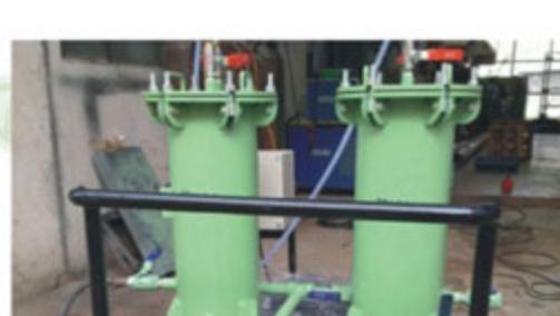
Portable Hydraulic filtration unit
